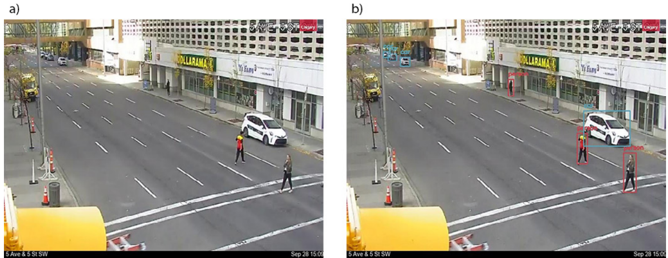
Figure 6 Example of detecting pedestrians in the city of Calgary a) before object detection and b) after object detection
